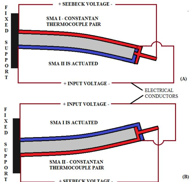
**FIGURE 13.** ACTUATOR-SENSOR CONFIGURATIONS USING SMA LAYERS AND CONSTANTAN
