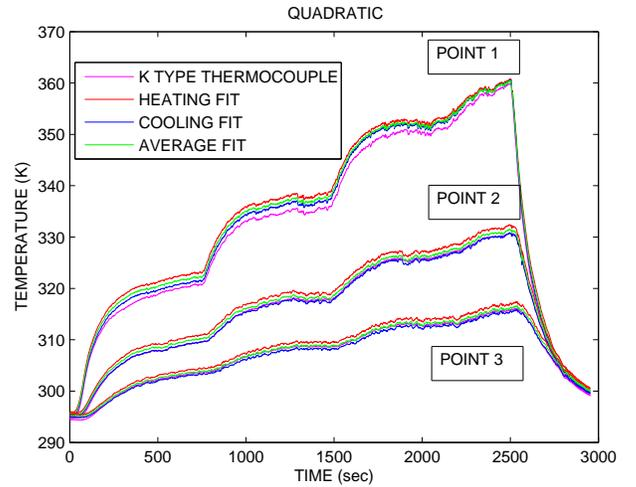
**FIGURE 7.** K-TYPE THERMOCOUPLE AND QUADRATIC FIT FOR VALIDATING THE SEEBECK VOLTAGE - TEMPERATURE RELATION
