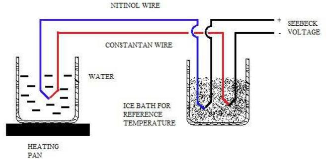
FIGURE 2. EXPERIMENTAL SETUP FOR SEEBACK VOLTAGE CHARACTERIZATION
