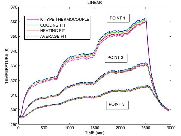
**FIGURE 6.** K-TYPE THERMOCOUPLE AND LINEAR FIT FOR VALIDATING THE SEEBECK VOLTAGE - TEMPERATURE RELATION
