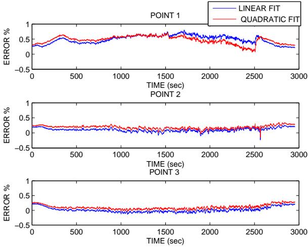
**FIGURE 8.** COMPARISON OF ERROR % BETWEEN LINEAR FIT AND QUADRATIC FIT
