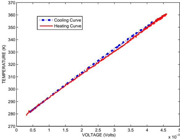
**FIGURE 3.** THERMOELECTRIC VOLTAGE vs TEMPERATURE
