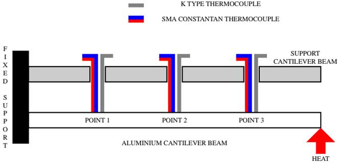
**FIGURE 5.** EXPERIMENTAL SETUP FOR VALIDATION OF SEEBECK VOLTAGE RELATION
