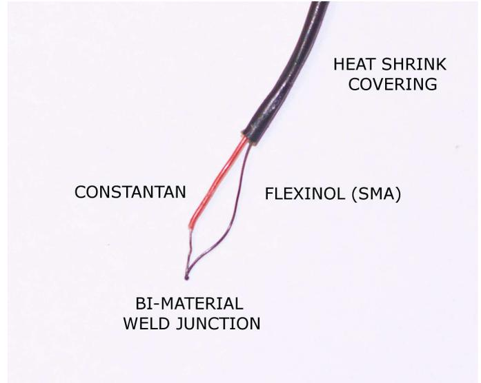
FIGURE 1. FLEXINOL(SMA)-CONSTANTAN THERMOCOUPLE
